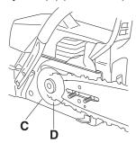
The front hand guard is not designed solely to activate the chain brake. Another important feature is that it reduces the risk of the chain hitting your left hand if you lose grip of the front handle.
